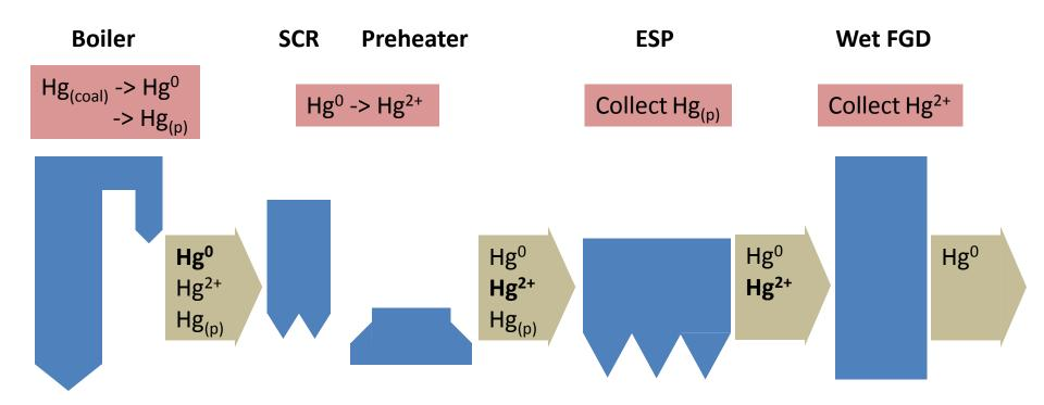
Processes across multiple units that are largely unengineered and uncontrolled for Hg
