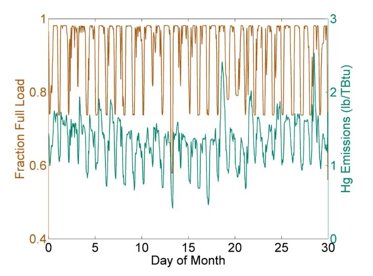
Load affects downstream AQCS; likely Hg oxidation in SCR
