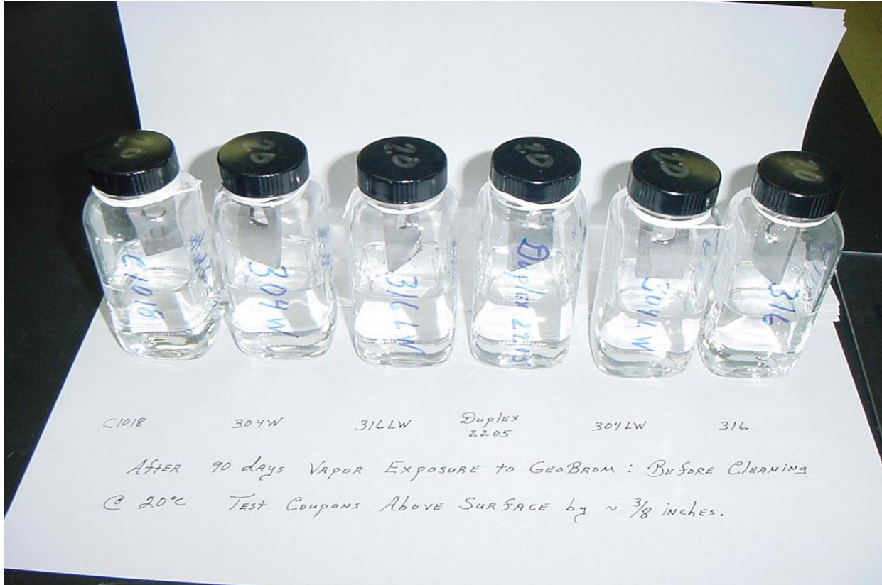
Figure #3 → Test Coupons after 90 day Above Surface exposure at 20° C and 50° C while still in Test Bottles (before cleaning)
