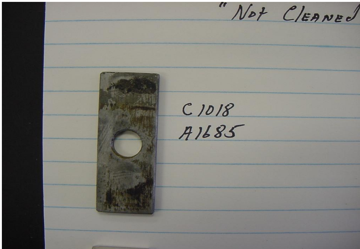
Figure #8 → Back side of C1018 Test Coupon after 90 day subsurface exposure at 50° C (before cleaning)
