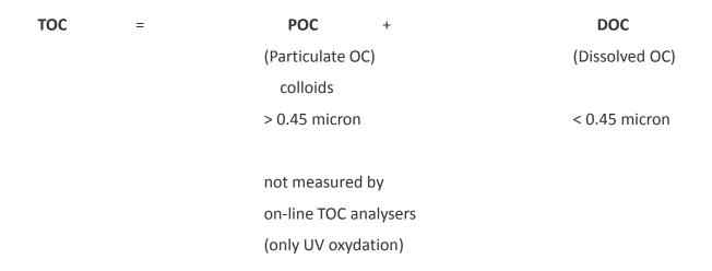
Often the driving factor for selecting the correct boiler water make-up plant process.
