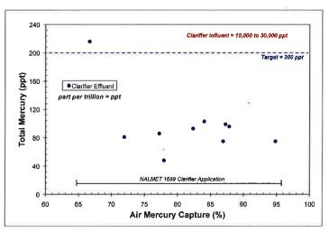
Figure 2 - NALMET 1689 Control of Wastewater Mercury Concentrations
