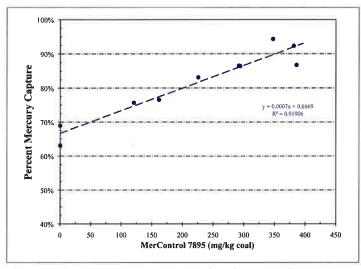
Figure 1 - Gas-Phase Mercury Removal performance Curve
