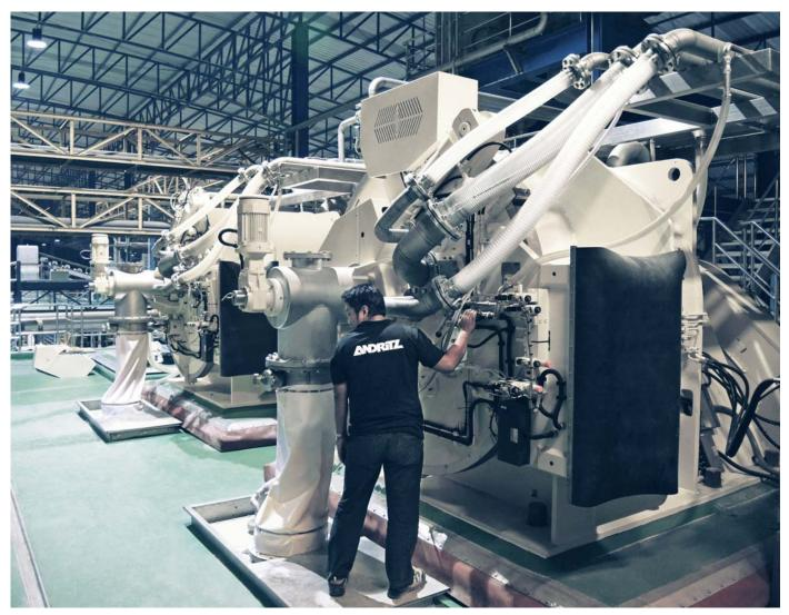
ANDRITZ delivered three fully automated Krauss-Maffei peeler centrifuges to a tapioca starch project in Thailand which were designed specifically to reach the same previous performance as up to 20 manual centrifuges.
