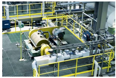
In the chemical industry, regular shutdowns of the process are required to seal the decanter casing again. Investing once in an innovative upgrade product (FRP – Fiber Reinforced Plastic decanter casing) by ANDRITZ can solve the issue with wear and downtime.
