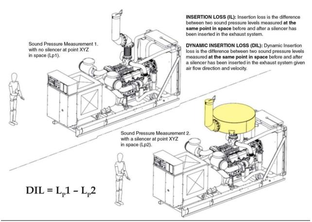
Figure 1 Dynamic Insertion Loss (DIL)
