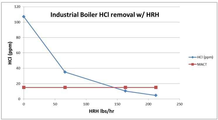
• HCl control to below MACT levels with High Reactivity Hydrate
