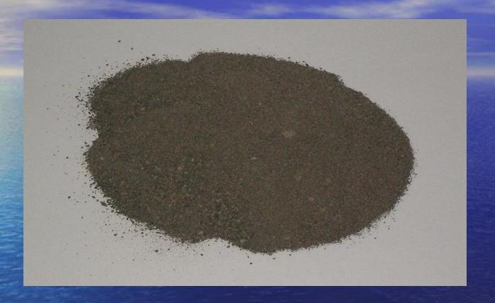
Particulates Contain Mercury and can also Filter Mercury from the Sample Stream
