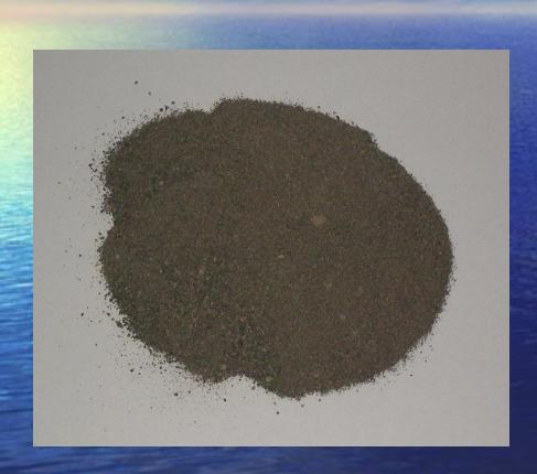
**Elemental Mercury Vapor** was Introduced to a Series of Blank Sorbent Traps with an Additional Section **Added Containing** Particulates from a Test Source. All the Mercury Passed through the Particulates and was **Recovered on the First Charcoal Section of the** Traps.
