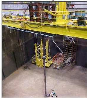
Shaft run-out test at bottom of 750,000 gallon test tank.
