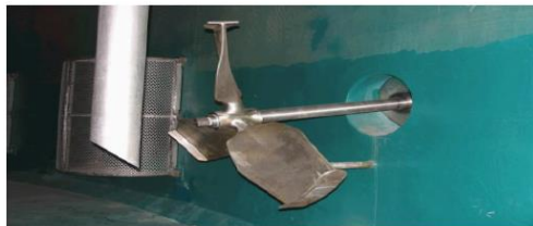
Fig. 9 Agitator and Air Lance
